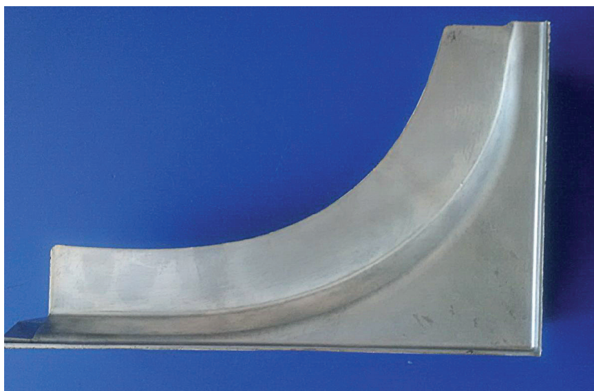
Thin-walled structural component made of a high-strength Silafont-38 alloy tested at G. A. Röders in a practical casting test (Photos and Graphics: Rheinfelden Alloys)
